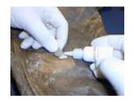
bring all surfaces even and smooth. It may be necessary to shave the insert by using a razor blade to remove any high areas from the surface that may still exist. Once this has been completed, clean the area once again to remove all particles and residue from the area and proceed to the next step.
